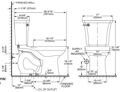
THIS TOILET IS DESIGNED TO ROUGH-IN AT A MINIMUM DIMENSION OF 305MM (12") FROM FINISHED WALL TO C/L OF OUTLET. SUPPLY NOT INCLUDED WITH FIXTURE AND MUST BE ORDERED SEPARATELY. \* DIMENSION SHOWN FOR LOCATION OF SUPPLY IS SUGGESTED.
